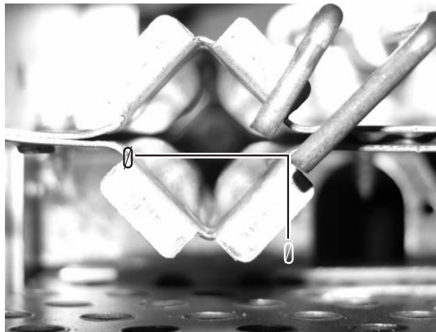
FIGURE 43 UPFLOW OPTIMUM IGNITOR LOCATION
